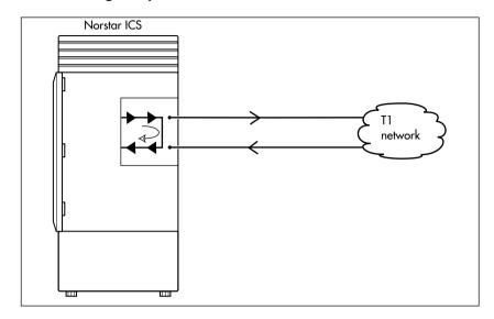
The card edge loopback test loops the outgoing signal on the DTI back to its internal received signal path. Signal paths to the external network are disconnected.
