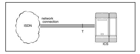
A T loop can be used in combination with an S loop to provide D-packet service for a point-of-sale terminal adapter (POSTA) or other D-packet device. D-packet service is a 16 kbps data transmission service that uses the D-channel of an ISDN line.
