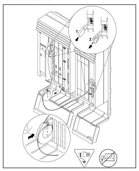
The cable trough can accommodate two fibre cable spools. Either slot may be used.
