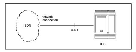
U-NT and U-LT loops can be used in combination to provide D-packet service for a point-of-sale terminal adapter (POSTA) or other D-packet device. D-packet service is a 16 kbps data transmission service that uses the D-channel of an ISDN line.
