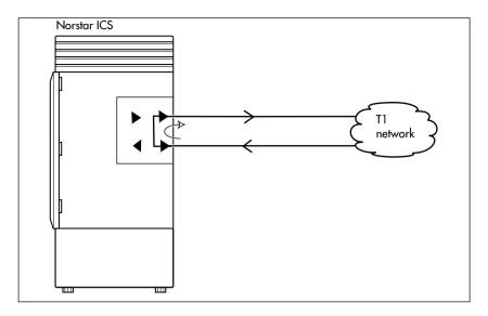
The line loopback test loops the full 1.544 Mbps signal received from the network back to the network. The looped signal is regenerated without any change in the framing format and without the removal of any bipolar violations. The line loopback test can also be invoked and stopped remotely using the in-band signal or via the facility data link (FDL) in extended super frame (ESF) format.
