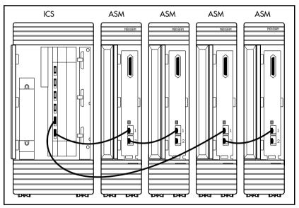
After the modules are mounted and connected, feed the cables through the cable trough.
