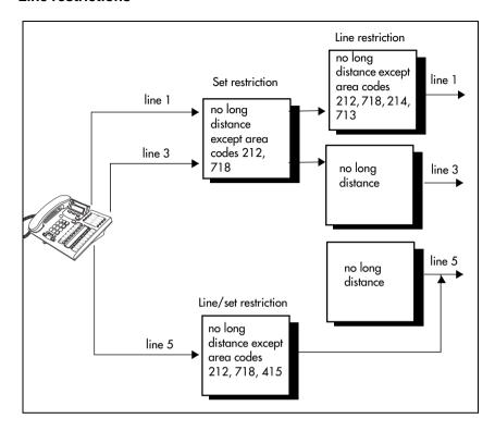
In the previous diagram, a caller using line 1 could only dial long-distance numbers to area codes 212 and 718. A caller using line 3 could not dial any long-distance numbers. A caller using line 5 could dial long-distance numbers to area codes 212, 718, and 415.
