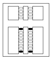
If you just want to cold start an individual module, on that module, simultaneously press the two top and two bottom buttons on the lower button set, as shown in the following diagram. The KIM displays a random pattern of icons as the KIM resets
