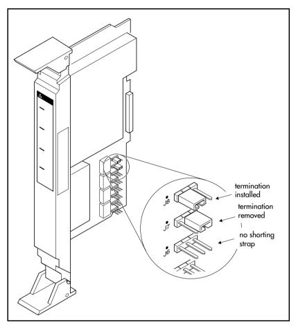
Ensure that the shorting straps are installed on both the receive and transmit jumpers for the loop. Refer to the illustration above.
